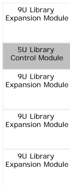
**Warning:** All libraries taller than 14U must be installed in a rack having a main protective earthing (grounding) terminal, and power must be supplied via an industrial plug and socket-outlet and/or an appliance coupler complying with IEC 60309 (or an equivalent national standard) and having a protective earth (ground) conductor with a cross sectional area of at least 1.5 mm<sup>2</sup> (14 AWG).
